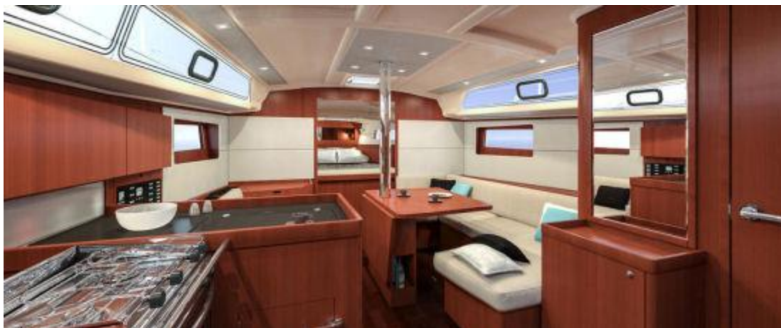
The L-shaped galley to port. Notice the abundance of windows, both above and below the gunwale, allowing an abundance of natural light to enter the salon.
