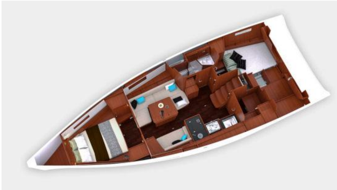
Plan view of the Oceanis 41.1 in the two stateroom, single head configuration.
