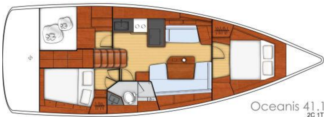
The twin cabin with a port quarter storage locker and single head configuration.
